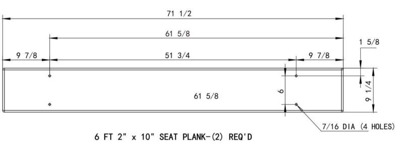
\*Dimensions provided are for reference only. Please verify measurements directly with the frame before drilling.
